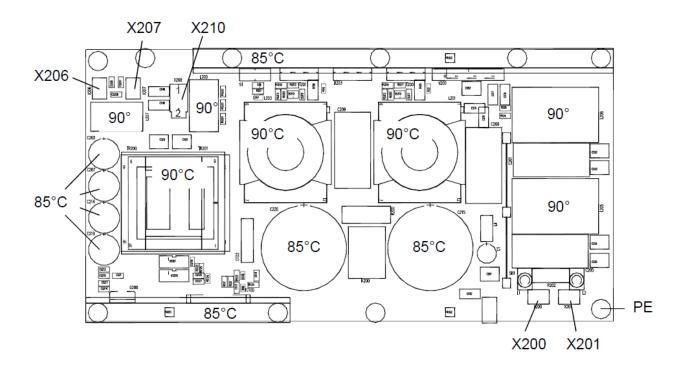
All points in the drawing marked with PE must be connected to protective ground
