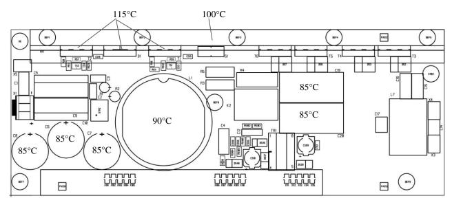
The temperatures specified above are maximal values. Exceeding the stated temperature values for capacitors leads to reducing the service life.
