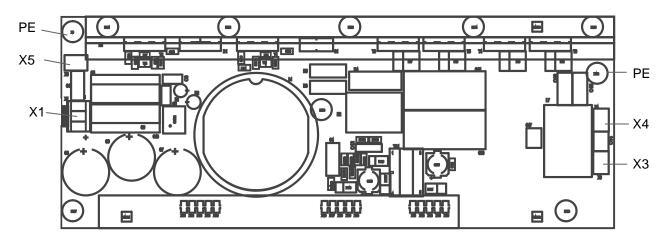
All points in the drawing marked with PE must be connected to protective ground
