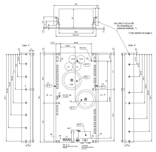
The temperatures specified above are maximal values. Exceeding the stated temperature values for capacitors C2 and C3 leads to reducing the service life.
